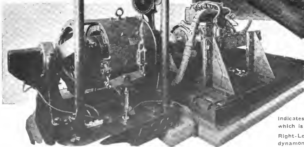
Above—Control features of Zenith testing laboratory. A , automatic switch which cuts in when double throw switch D is swung to dynamometer position. F is the field rheostat and the wheel F is hand control for same. W is the switch starting the dynamometer as a motor. S and T are spark and throttle controls. I is the Ignition switch, M the tachometer and V indicates the voltage of the transformer set, which is adjusted by rheostat R .
